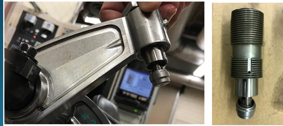
Cylinder-deactivation through Eaton's collapsible lifter
