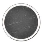
**Test Conditions** – Test Cycle: UDDS (Urban Dynamometer Driving Cycle; Test Distance: 5.5 miles over 17 minutes; Fuel Consumed during the Test: 1.1 gallons; Test Vehicle: Heavy-duty truck with a 370 hp Cummins engine (1999 model year).
