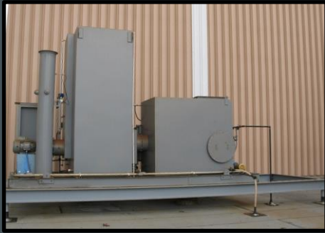
Pilot Scale Fiberbed Mist Collection System
