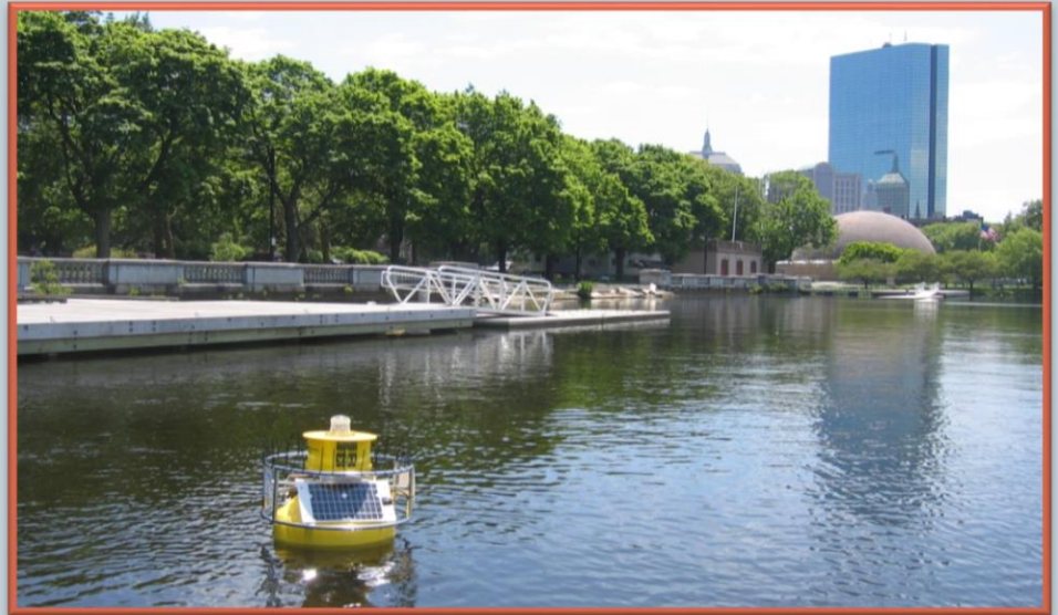
Monitoring buoy in Charles River collects and transmits data
