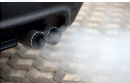
Figure DF-14: Example of White Smoke from Tailpipe
