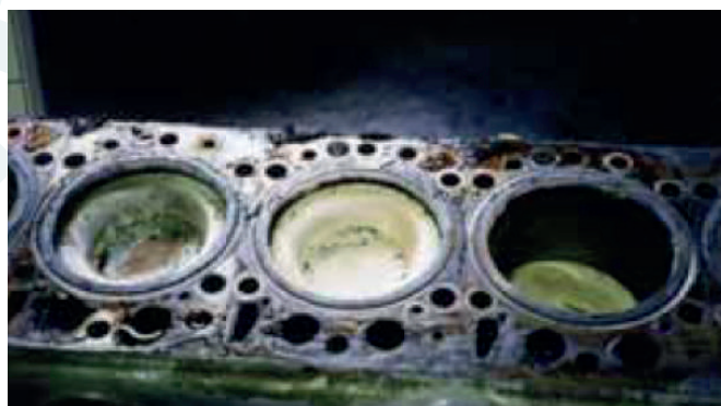
Figure 10: Picture of an Engine Damaged by Silicon
