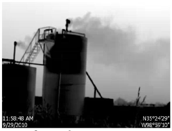
**Infrared Camera Use for VOC Inspections**
