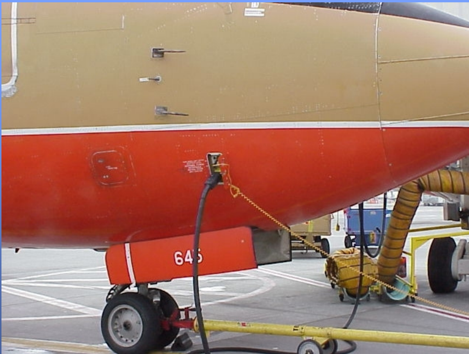
Electric Power to Southwest Plane at Sac Metro
