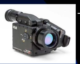
The infrared gas-imaging camera consists of a modified Indigo (FLIR/Indigo Systems Corp., Goleta CA) Merlin MID camera with a nominal spectra range of 1-5.4 micrometers
