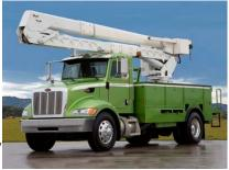
vehicle from a stop. Lithium-ion batteries operate the PTO unit, which is designed for municipal and utility applications. Both of the medium-
